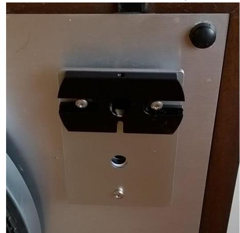
**Step 5;** Screw in but don't tighten. (Three screws)
