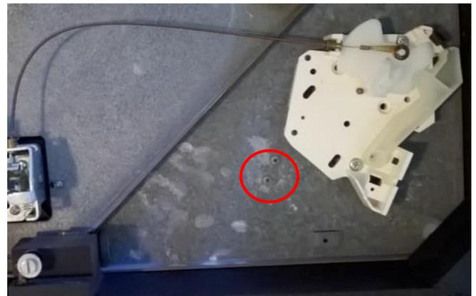
**Step 7;** Turn over and remove the arm. (Three screws)
