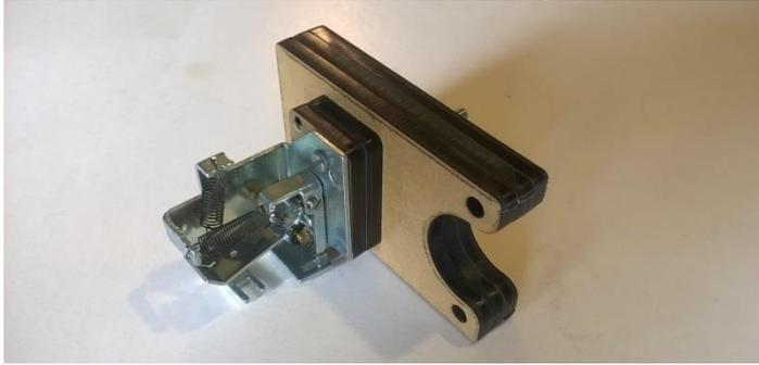
**Step 2;** Screw through the lifter mechanism with two long screws.
