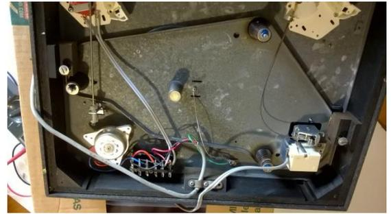
**Step 3;** Remove the arm cable clamp and the white cable cover.
