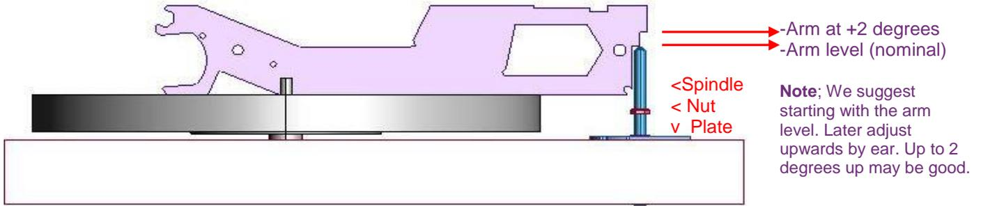
**Step 2;** Position the mount using the protractor (Slide back and forth)
