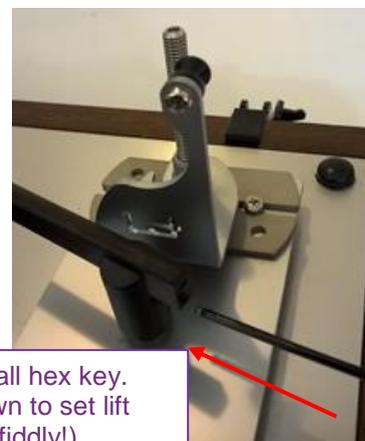
Lock with small hex key. Slide up / down to set lift Height (very fiddly!)
