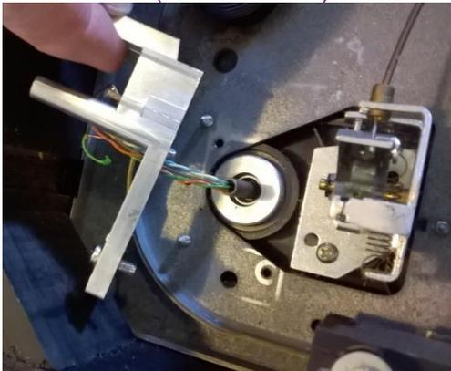
**Step 6;** Remove the armrest (two screws)
