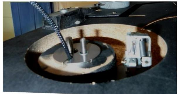
**Step 3;** Feed wire through slot in plate
